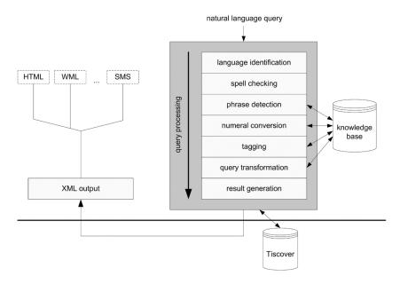
Figure 1: Software Architecture
