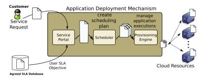
Figure 5. Application deployment mechanism. SLA, service level agreement.
