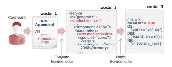
Fig. 11. Delegation of service parameters used for deploying VM products in the Genomics use case
