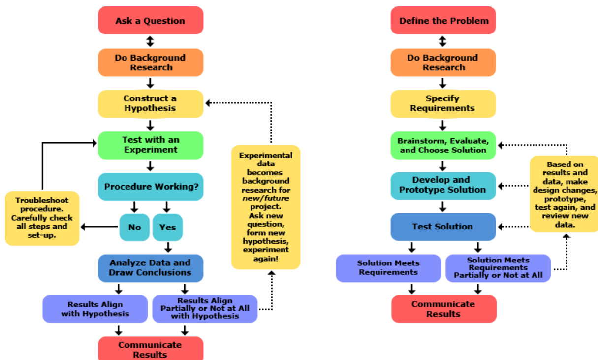
Figure 1 Scientific method (left) vs engineering design process (right) [1]
